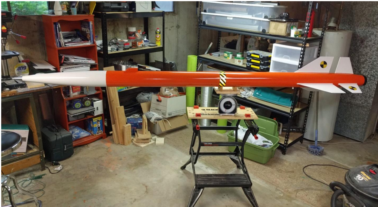
Weighing and balancing the rocket for refinement of the simulation.
