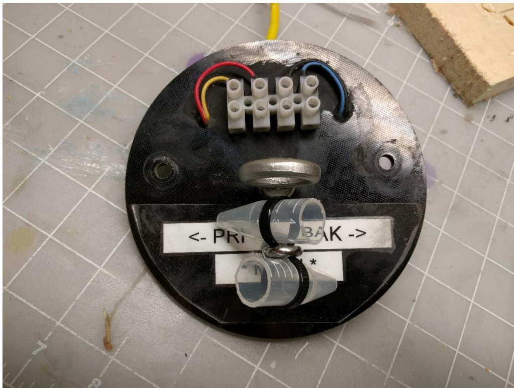
Detail of outside of electronics bay bulkhead, showing terminals for attaching deployment charges and eyebolt for supporting charge canisters.
