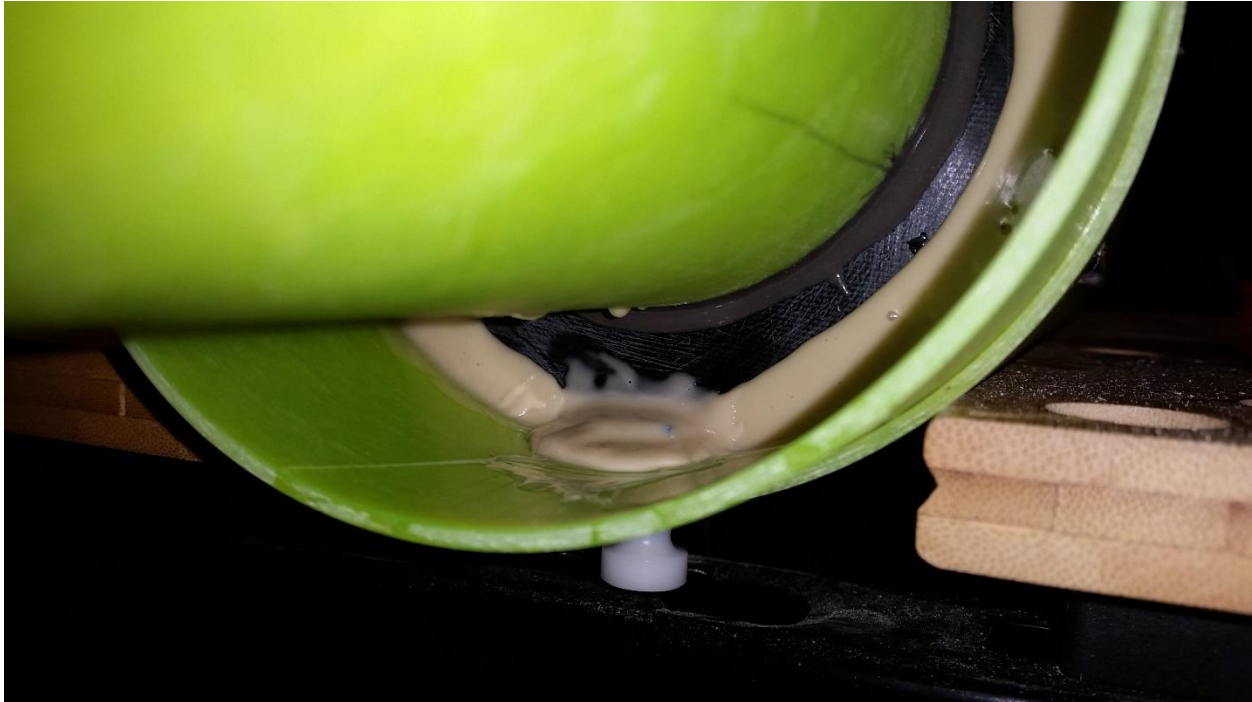
Detail of rail button backing T-nut bonded to airframe and centering ring.
