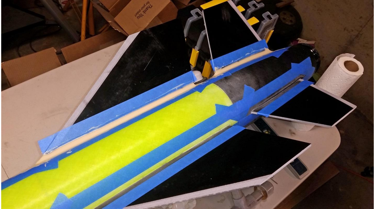
Application of external fillets.
