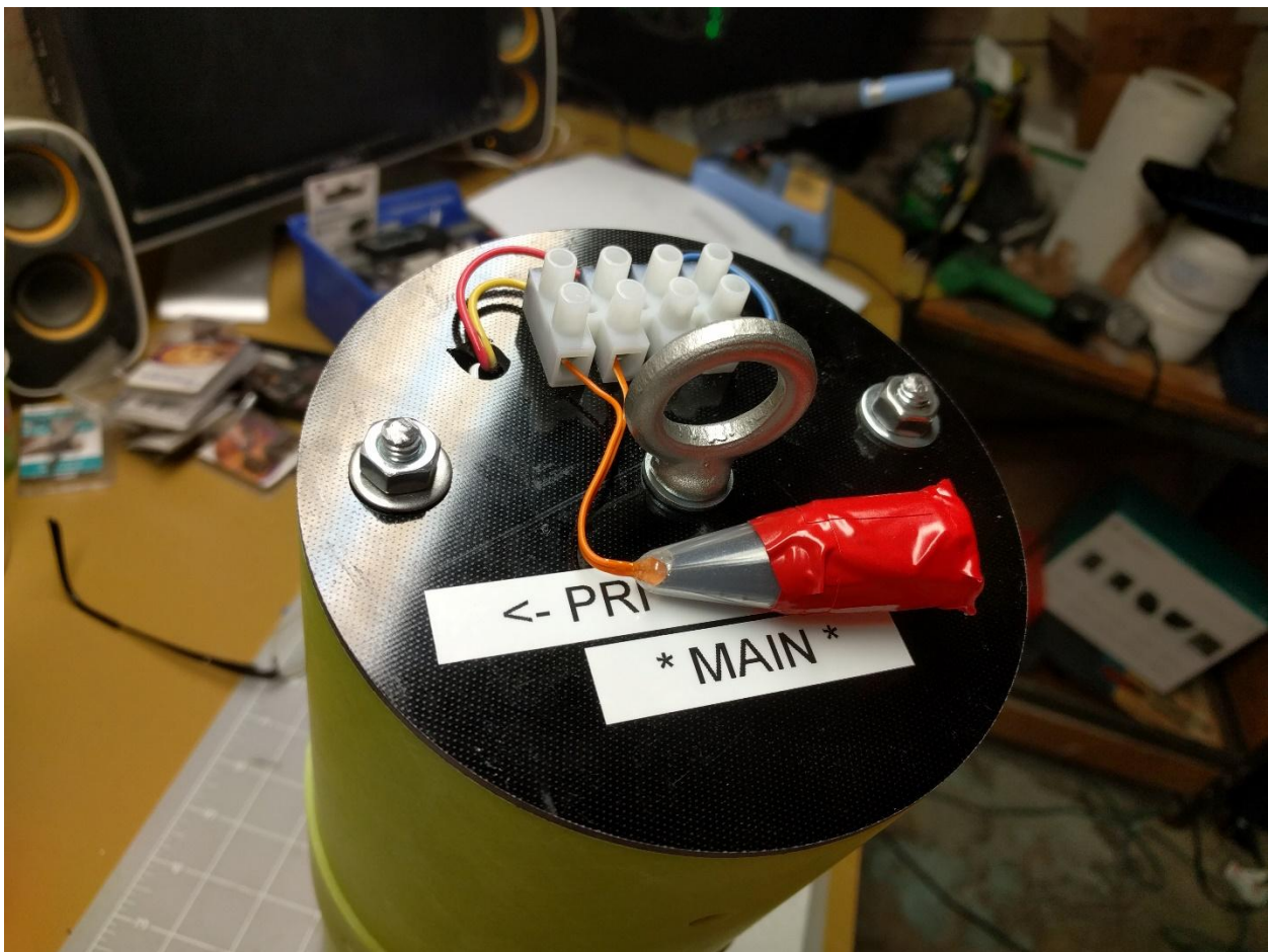
Ejection charge connected to terminal block for ground test. (Not shown: zip-tie support for charge canister.)
