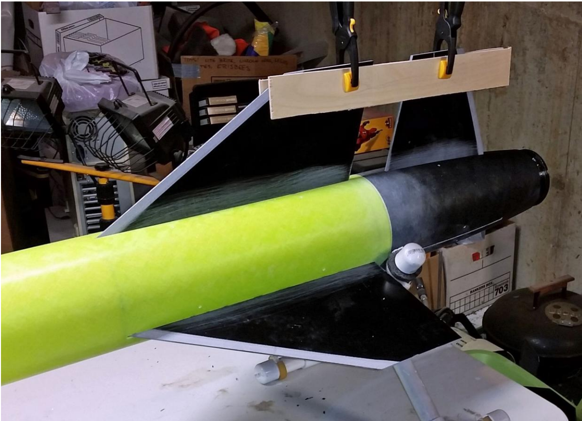
Initial bonding of aft fins; plywood alignment strips shown.
