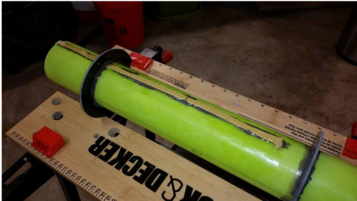
Recovery system anchor bonded to motor mount tube. (Also bonded on opposite side of tube.)
