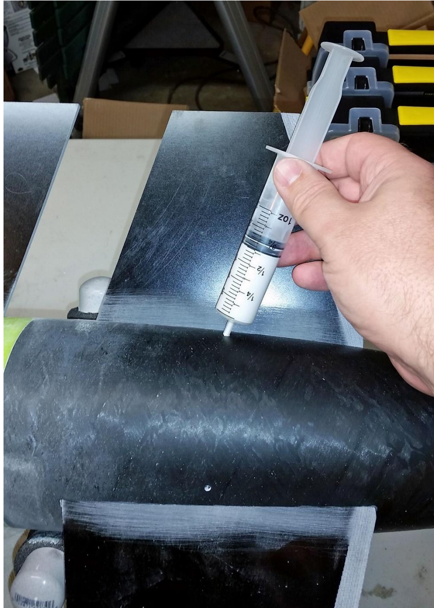
Injection of internal fillets.
